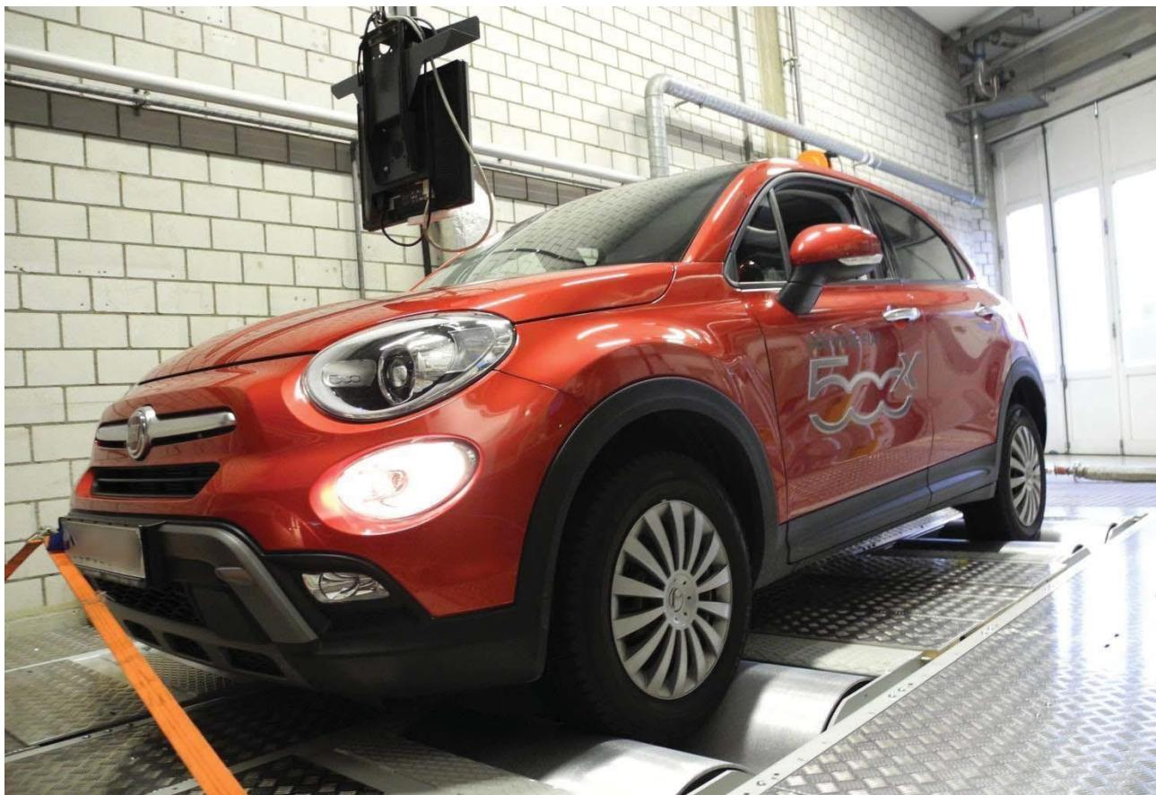
Fig.1: Fiat 500x 2.0 MJ on the 4WD dynamometer at the exhaust emission control lab
