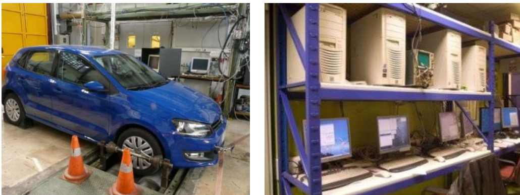
Figure 6: LAT chassis dynamometer (left) and chassis dynamometer control station (right)
