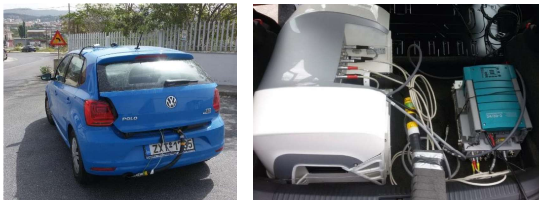
Figure 1: PEMS installed on the VW Polo (left) – PEMS and control module (right)
