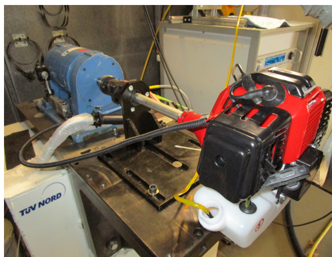
Clamping fixture for string trimmers/brush cutters.
