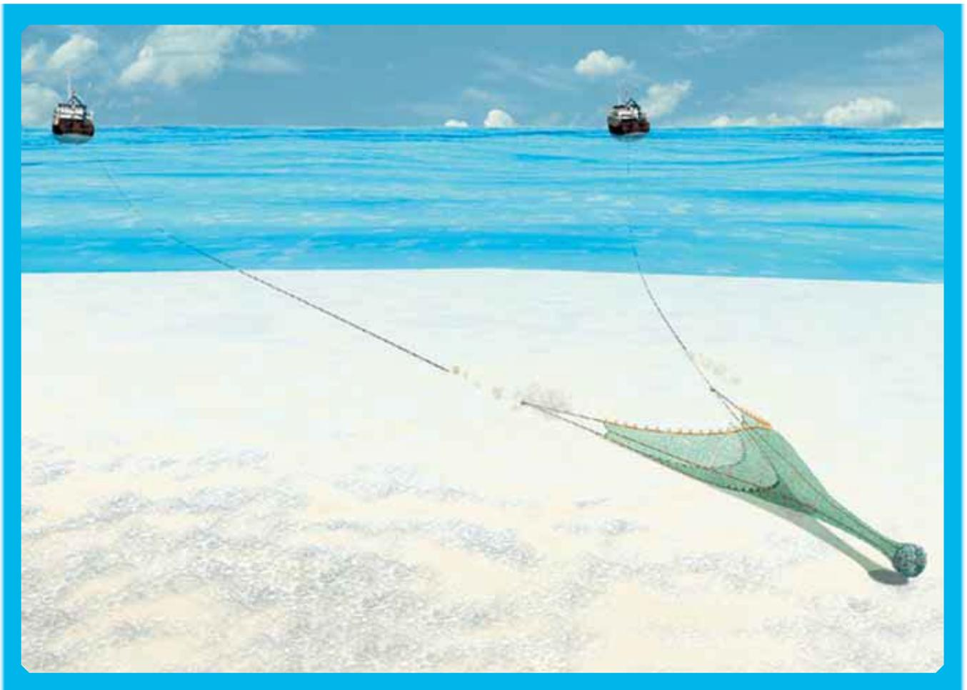
Abb. 23: Grundtuckschleppnetz (Illustration by Alvan Rice, © Crown Copyright 2005 ([Link 7](#)))
