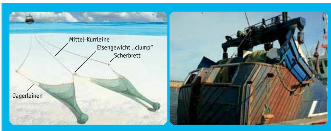
Abb. 24: *Twinrig* (Link 8) (© Crown Copyright 2005 (Link 7))
