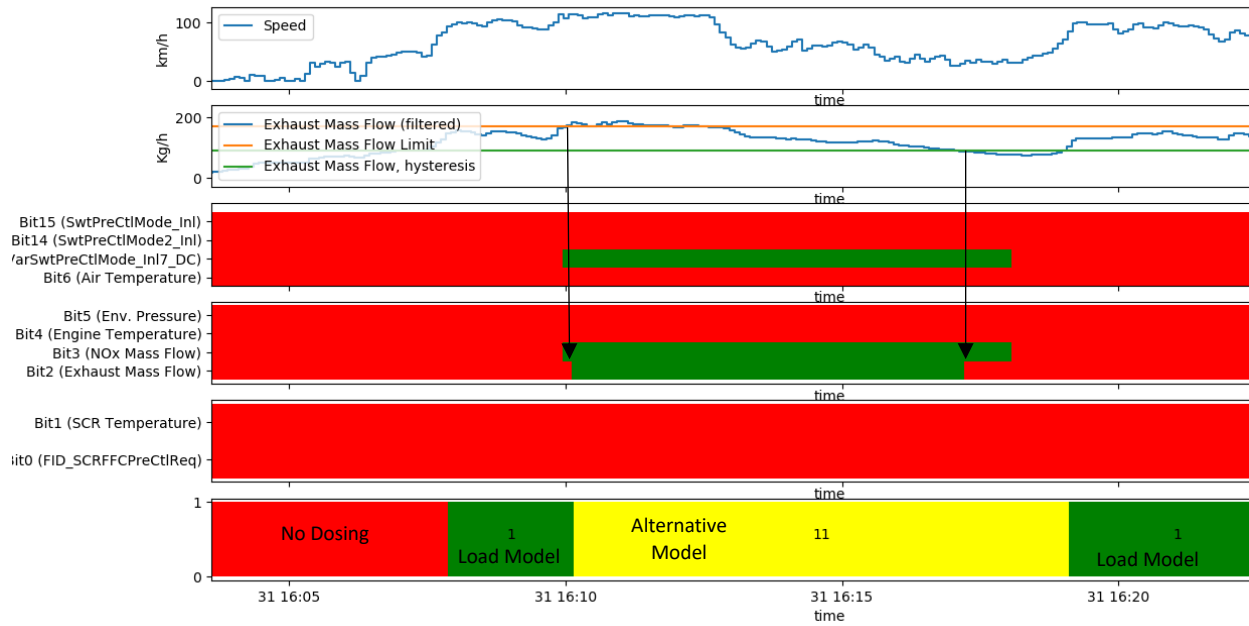
Figure 3 – Measurement data with original software; Two events visible: at around 16:10 (left black arrow), the exhaust mass flow exceeds the limit of 170kg/h, causing the defeat device to activate, enforcing a switch to the Alternative Model. At around 16:17 (right black arrow), the defeat device deactivates, eventually allowing a switch back to the Load Model. (Other defeat devices, for example the NO x mass flow limit, activate at the same time.) Bit names refer to the bit positions in the “prectI2”-Mode word that ECU software uses to determine when to switch to the alternative mode.
