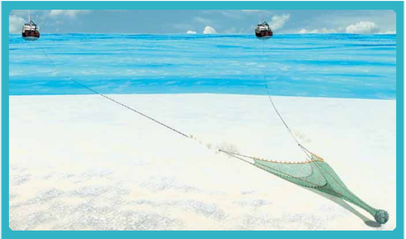
Abb. 23: Grundtuckschleppnetz (Illustration by Alvan Rice, Crown Copyright 2005, http://www.scotland.gov.uk/CrownCopyright )
