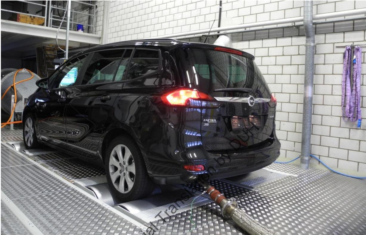
**Fig. 1:** OPEL Zafira CDTi 1.6 on the 4x4 roller dynamometer at the exhaust emission control lab
