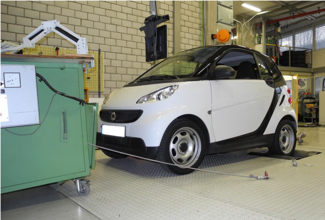
Fig.1: Smart fortwo coupe cdi on the roller test bench at the exhaust emission control lab
